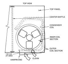
Fig. 10 - Separating Coil Sections
